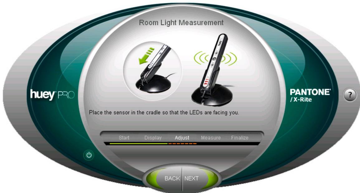
**Note:** The *ambient light sensor* is for adjusting your monitor’s contrast according to the room lighting conditions. This helps the display look the same as light changes throughout the day. The sensor measures the ambient light before profiling.
